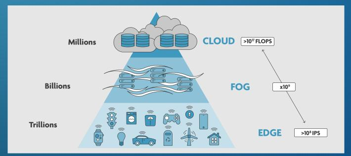
Fig. 2: Edge-to-Cloud information processing model for AI leads to unsustainable and inefficient zettabyte data movement (Source: EPFL View on Future Grand Challenges [A119]).
