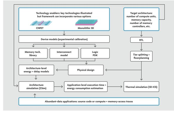
Fig 12: N3XT system-technology exploration environment for multicore processor systems [Aly19]
